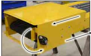
Fig 32 - S-Drive discharge roller belt treading
