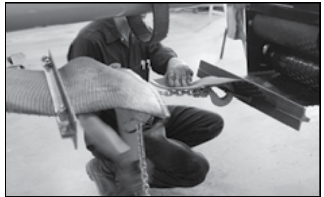
Fig 21 - Use a Come-Along Winch to pull
