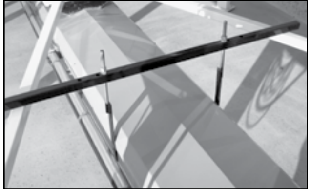
Fig 13 - Hanger bar with brackets bolted on
