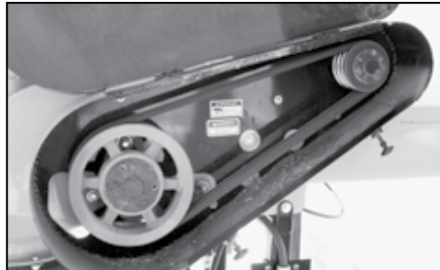
Fig 51 - Drive side with guard opened
