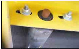
Fig 34 - Rollers are adjustable
