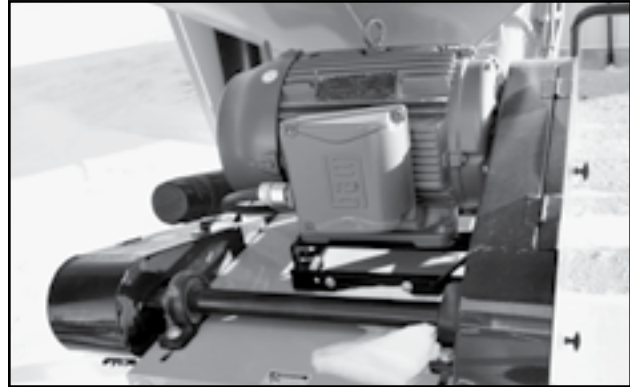
Fig 32 - Electric engine and drive assembly
