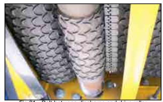
Fig 21 - Belt between discharge and drive roller
