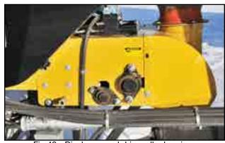
Fig 48 - Discharge and drive roller bearings
