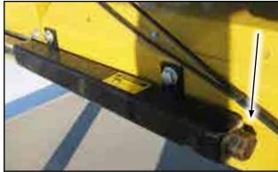
Fig 53 - End drive tensioning jacks
