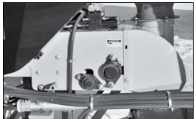
Fig 41 - Discharge and drive roller bearings
