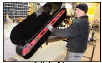
Fig 29 - Align Pulleys
