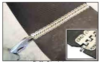
Fig 25 - Crimp lacing
