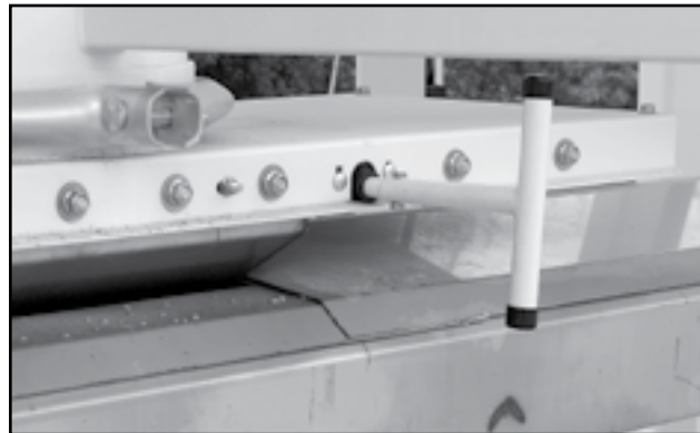
Fig 8 - Gate assembly with manual crank
