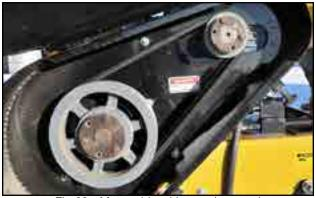
Fig 60 - Motor side with guard opened
