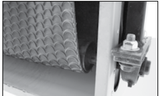
Fig 40 - Tail roller from underneath
