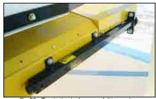
Fig 26 - Tensioning jacks on end drive system
