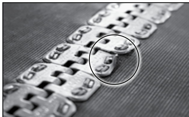
Fig 27 - Something catching on belt lacing
