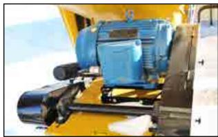
Fig 39 - Electric engine and drive assembly
