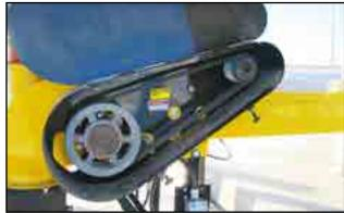
Fig 28 - V-belts and pulleys
