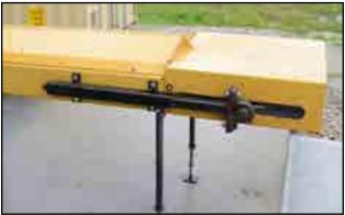
Fig 46 - Tensioning jack
