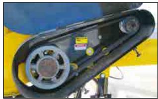
Fig 58 - Drive side with guard opened
